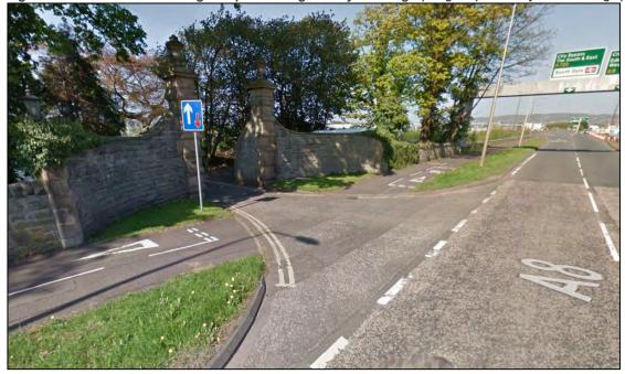
A distance of 9.8metres was measured between the stop line and the gate piers, indicating that 1 vehicle can be accommodated at the mouth of the access without causing obstruction to the traffic on the A8.
